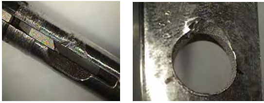
Fig.4 Breakage of tool tip (SM45C Wa=30°, 600rpm, f=30mm/min)
