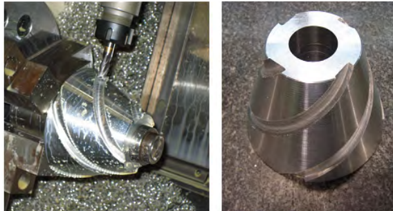
Fig. 8 5-axis NC machining using NC data generated by the E-POST
