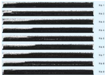
Fig. 4. Filling pattern of micro rib produced with reference condition
