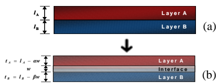
Fig. 3. Schematic diagrams for (a) simple and (b) expanded rule-of-mixture.
