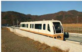
Fig. 3 Korea standardized rubber-tired light rail vehicle
