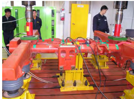
Fig. 1 Load test installation
