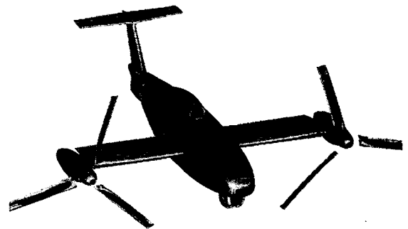
Fig. 1 A simply analyzed TR-S1 model of the Smart UAV
