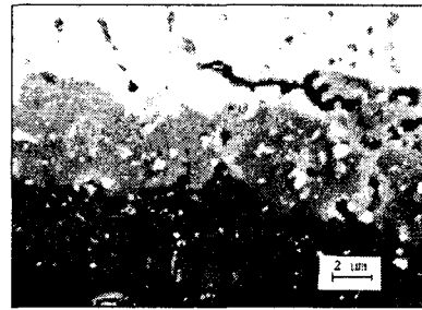
Fig. 9 Cross-sectional BEI of the oxidation products in the thermally cycled EB-PVD TBC
