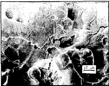
Fig. 1 SEM photomicrograph of the top surface of the as-plasma sprayed TBC
