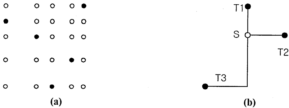
Fig.2 Hanan's grid graph and Steiner point for 3 Terminals
