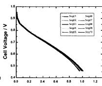
Current density / A cm<sup>-2</sup> Anode: 810 sccm H<sub>2</sub>, T<sub>A</sub>=105°C, p=30psig Cathode: 4000 sccm Air, T<sub>c</sub>=80°C, p=30psig Cell temp. = 80°C, 0.2 mg Pt/cm2 at each electrode
