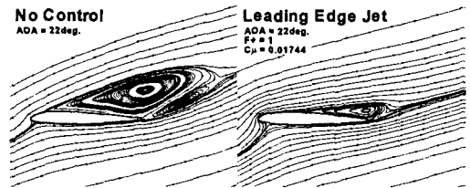
Fig. 3 Streamline at separation control on leading edge
