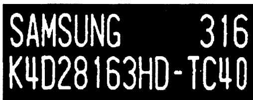
Fig. 3 Binary image using Otsu method
