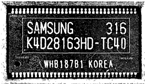
Fig. 2 Mark areas and template areas on chip
