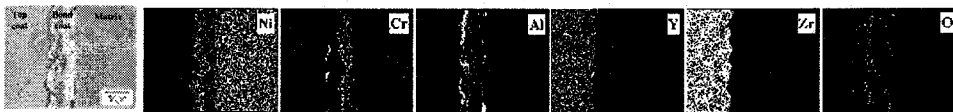
Fig. 2. Cross-sectional SEM image and elemental distribution of modified Inconel 713LC corroded at 675°C for 216 hrs (bond coat-NiCrAlY & aluminizing, top coat-YSZ).
