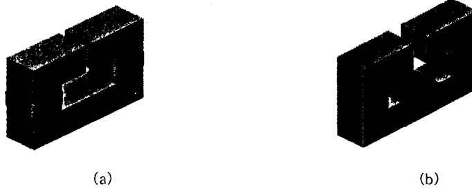
Fig. 1. Constructed (a)permanent magnet and (b)electromagnet system used for the magnetic field distribution measurement.
