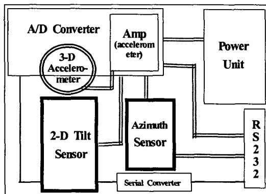
Fig.5 Hardware system of measuring device
