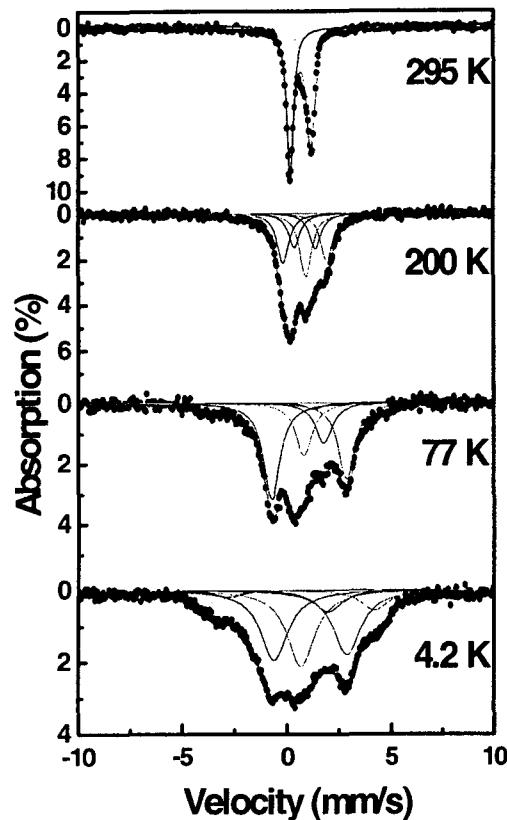
Fig.2. Mossbauer spectra of  $\text{FeCr}_2\text{Se}_4$  at various temperatures.
