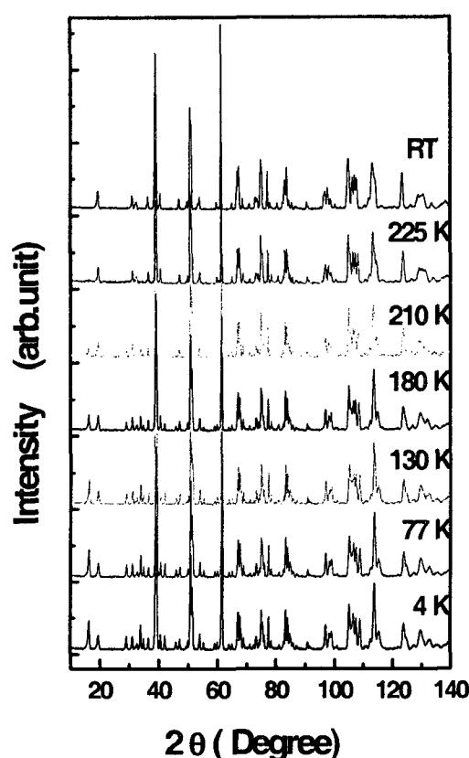
Fig.1. Neutron diffraction patterns of  $\text{FeCr}_2\text{Se}_4$  at temperature ranging from 4.2 to 295 K.
