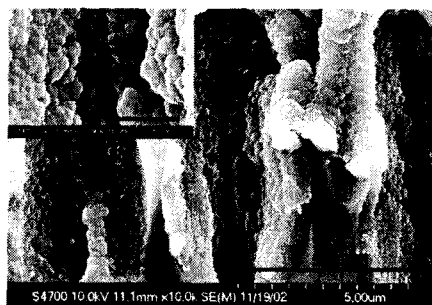
Fig. 3. SEM images for the cross-section of a PS-based urea sensor
