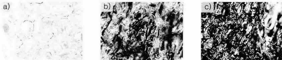
Fig. 1. Morphology of PIR foam
