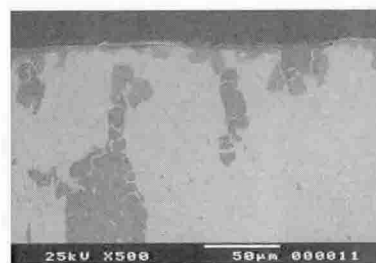
Figure 2. Photograph of the back-scattered electron image of the dispersion type (U-10wt%Zr)-50wt%Zr fuel/HT9.
