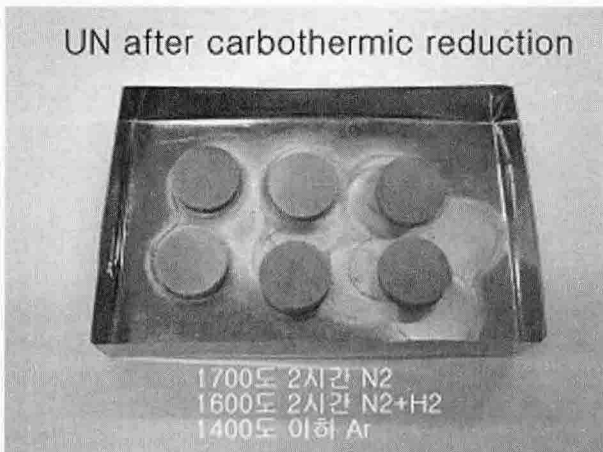
Figure 2. Nitride pellets after carbothermic reduction treatment.
