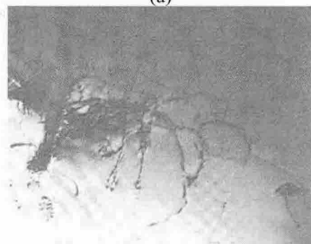
Fig. 2 Dislocations beneath the surface of fatigue fractured specimens of (a) LIS (b) HhL
