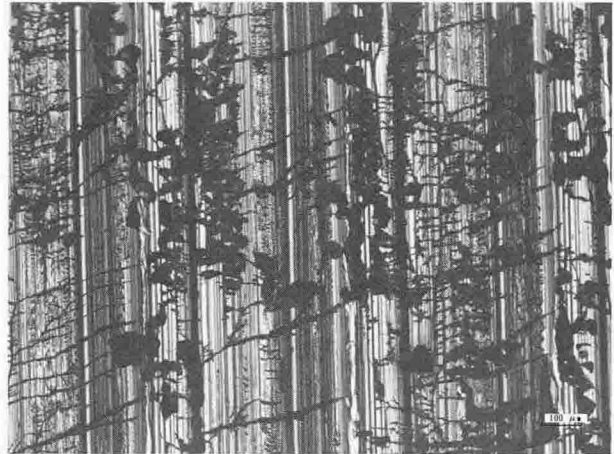
Figure, It shows a typical CWSCCs of 10 5 /cm 2 after the test on the cold-worked low carbon stainless-steel sample.
