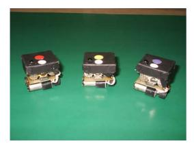
Fig. 7 Micro robots with color marks.
