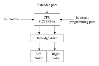
Fig. 4 Structure of control circuit.
