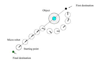
Fig. 10 Moving pattern of micro robot for gathering the object.
