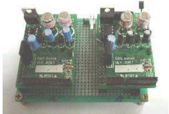
Fig. 5 Measurement board for sensor fault diagnosis.
