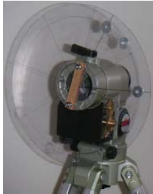
Fig.3 A rotator, remodeling of an equatorial telescope: The rotation speed is controlled by PC. The transparent plastic disk is rolled around the equatorial axis, where samples are set on the disk.
