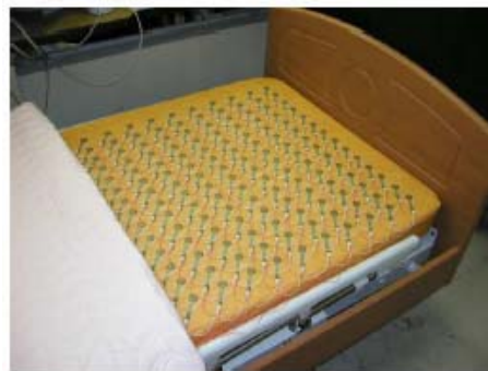
Fig. 4 Pressure sensors distribution bed.
