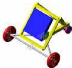
Fig 1. A basic model of 3 wheel based mobile robot.
