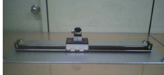
Fig. 11 3D active camera system
