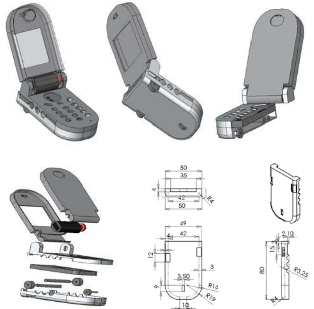
Fig. 12 The Mechanical System Design of RCP Prototype
