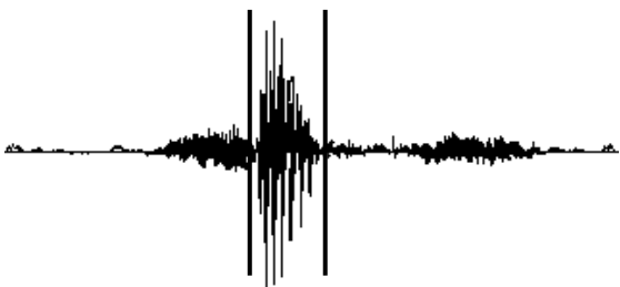
Fig. 2a The initial boundaries of six30.wav using rms energy in initial endpoint detection.
