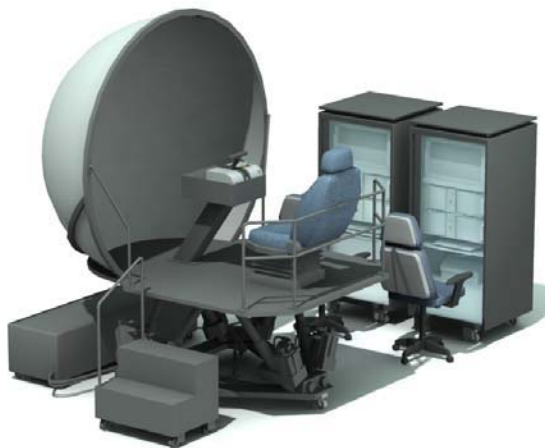
Fig. 13 The constructed driving simulator.
