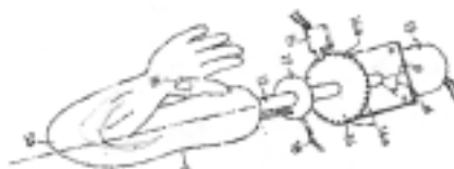
Fig. 5 Muscular force strengthening device for arm wrestling (JP 2002017891)
