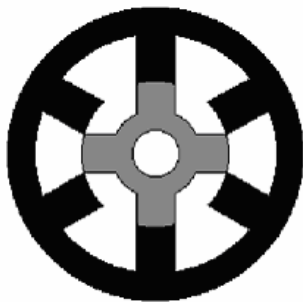
Fig 2 6/4 Switched Reluctance Motor
