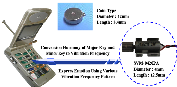
Fig. 10 Experiment of Emotion-Vibration Module
