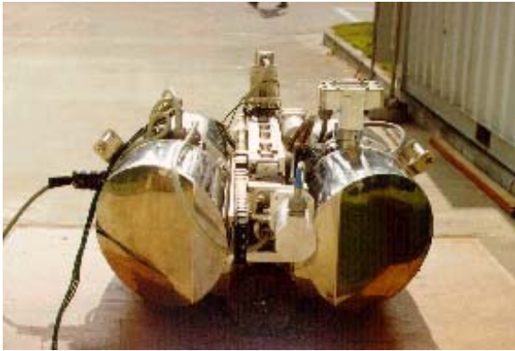
Fig.2 Reactor Inspection Robot (RIROB)
