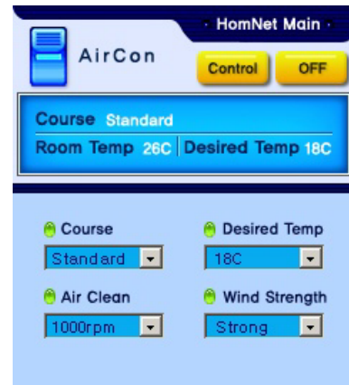
Fig. 8 The control page for air-conditioner
