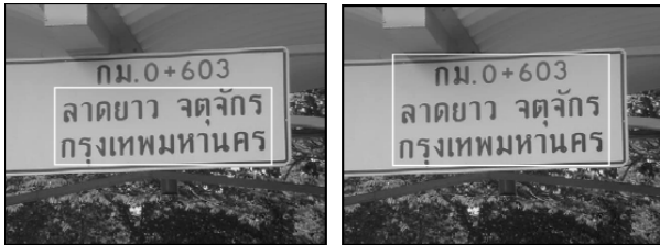
Fig. 8 A fault detection results due to using inappropriate kernel size (left) comparing to the one using the right kernel size (right).
