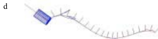
Fig.8 (a) A loop-like trajectory induced by large rotation angles damages the workpiece, (b) the trajectory simulated by the VMM, (c) the actual "repaired" trajectory, (d) the simulated repaired trajectory.
