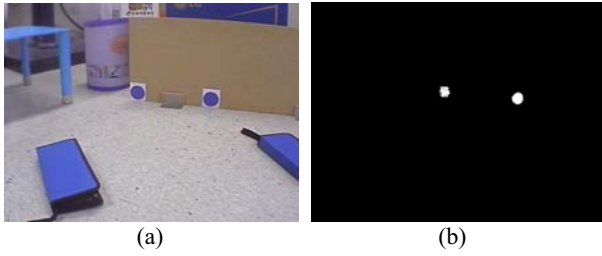
Fig. 2 Image Processing result for detecting the landmark: (a) before the image processing for detecting the landmark, (b) after the image processing for detecting the landmark.
