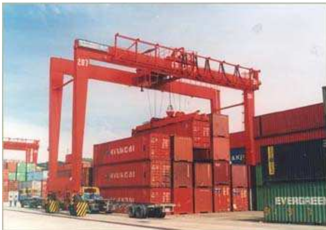
Fig. 1. Typical gantry crane used in container terminal.
