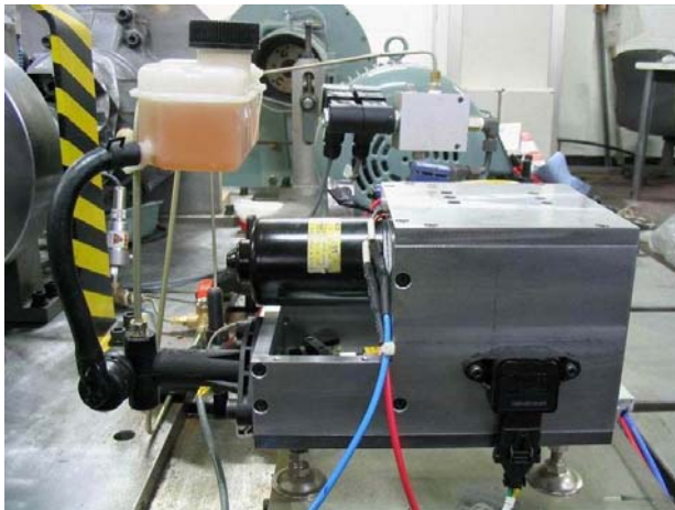
Fig. 5 Prototype of electro-mechanical type actuator
