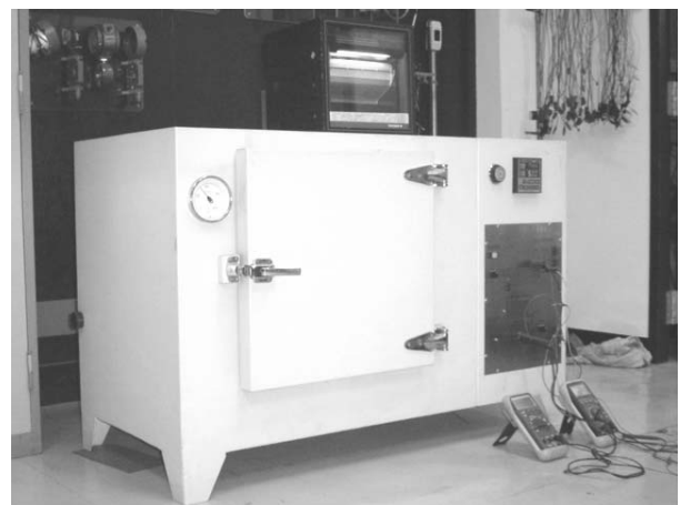
Fig. 6 Temperature control plant model (oven).
