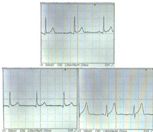
Fig.2. Measured ECG(oscilloscope view, channel 1, 2, 3)
