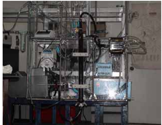
Fig. 3 Experimental circuit for the evaluation of oxygen transfers with bovine blood.
