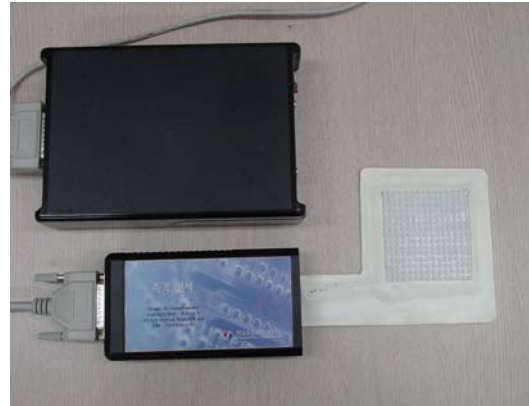
Fig. 3 A tactile sensor using FSR sensor(64 channels) and PVDF film(1 channel).
