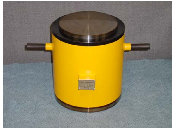
Fig. 1 10 MN load cell with column sensing element designed by KRISS.
