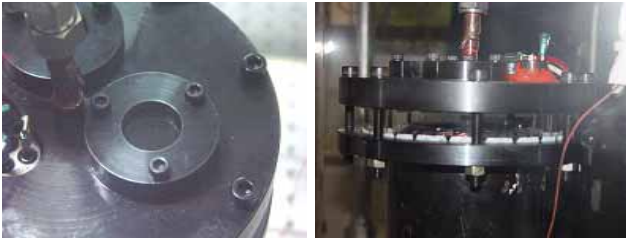
(a) Top view (b) Side view Fig.5 Photographs of rotary compressor with visualization windows
