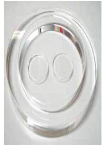
Fig.4 Quartz for visualization of rotary compressor
