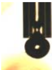
Fig. 4 Photograph of 'internal necking with attached bubble' regime for the nozzle of 1.55mm
