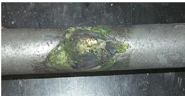
Fig. 3 Cracking as High Temperature Corrosion
