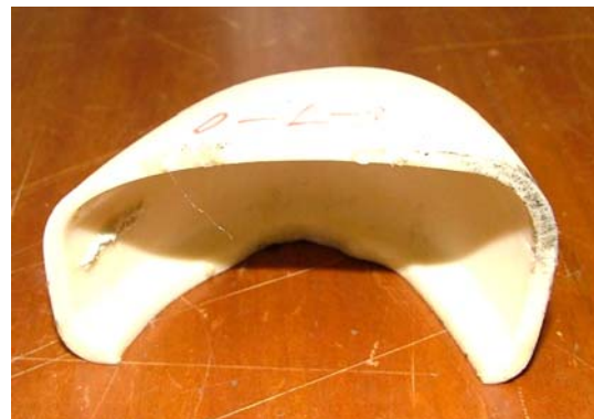
Photo 2 Modified Model of Toe-Cap After compression test
