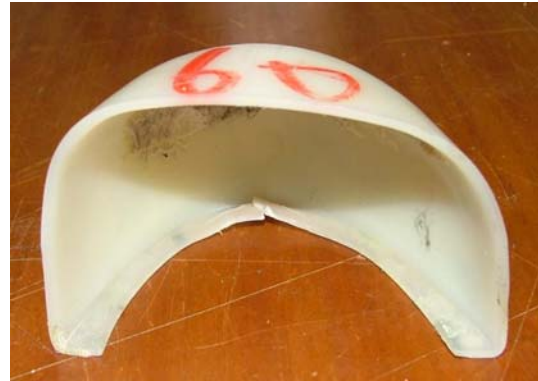
Photo 1 Initial Model of Toe-Cap After compression test
