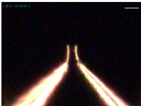
Fig. 6 Manufactured nanotweezer (scale bar : 5 μm)
